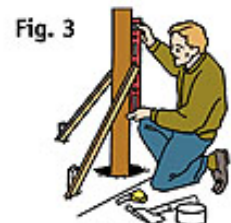
Use a level to make sure each post is in an exact, upright position.
